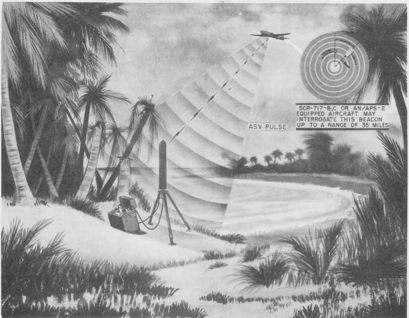
Radar Beacon AN/UPN-2 on being interrogated by airborne radar (on beacon function) replies in code permitting the beacon to be located in range and azimuth.
