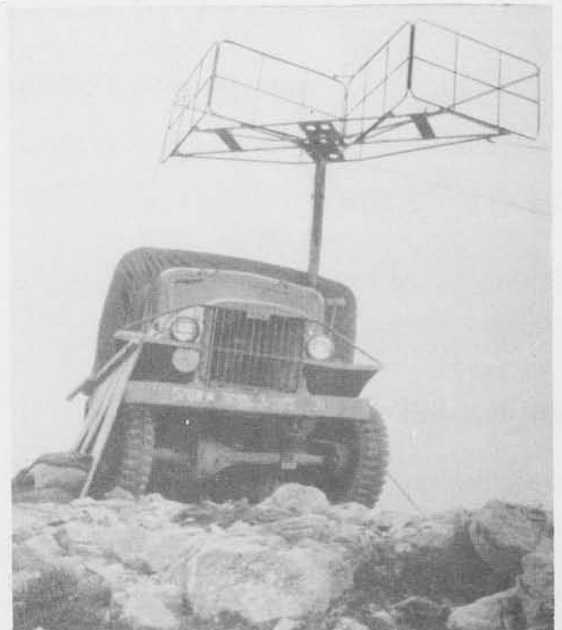
Radio set AN/CPN-2 should be placed on the highest terrain available and away from surrounding hills or buildings.
