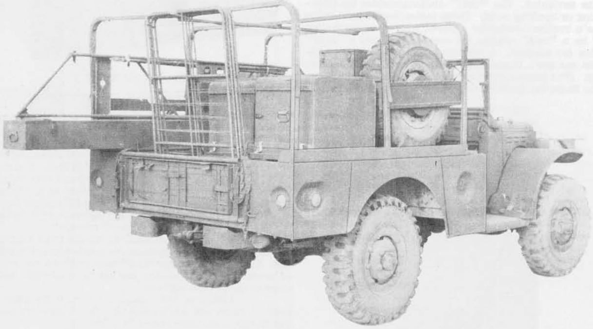
Complete installation of Vehicular Mounting Kit for Radio Set AN/CPN-2.
