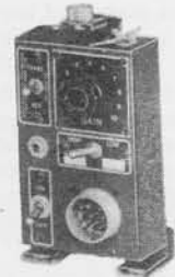
Control Box *C-3/APN-2 Mounting FT-406-A
