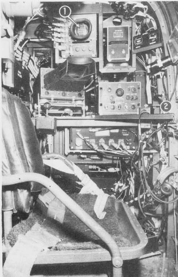
(1) Indicator BC-929-A (2) Radio Control Box BC-1145-A Radio Receiver and Transmitter BC-800-A (not shown) July 1945
