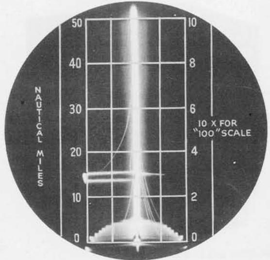
Scope records range vertically on three scales & azimuth horizontally right or left of centerline of beacon response signal above shows beacon 33 miles away & approx. 30° right.
