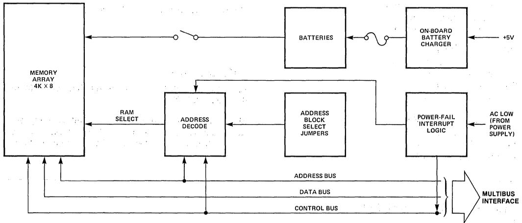
Figure 1. iSBC 094 Memory Backup Board Block Diagram
