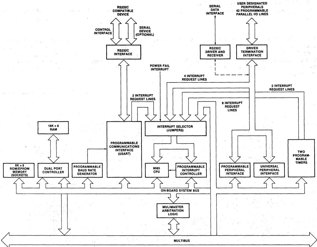
Figure 1. iSBC 80/30 Single Board Computer Block Diagram
