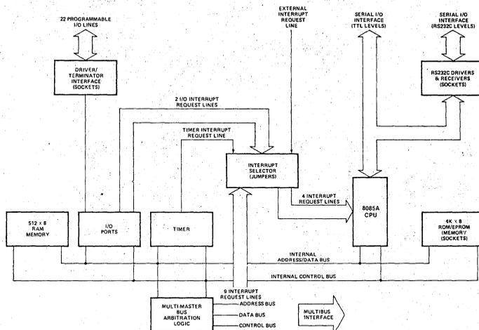
Figure 1. iIBC 80/05 Block Diagram Showing Functional Components
