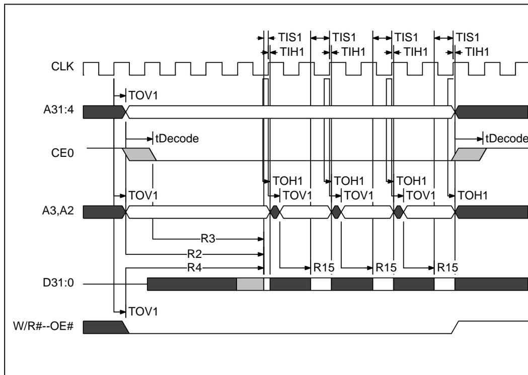
**NOTE:** The address line labels in this diagram refer to the labels on the i960 H CPU. Ax on the i960 H CPUs connected to Ax-1 on 3 Volt Intel® StrataFlash™ memory.
