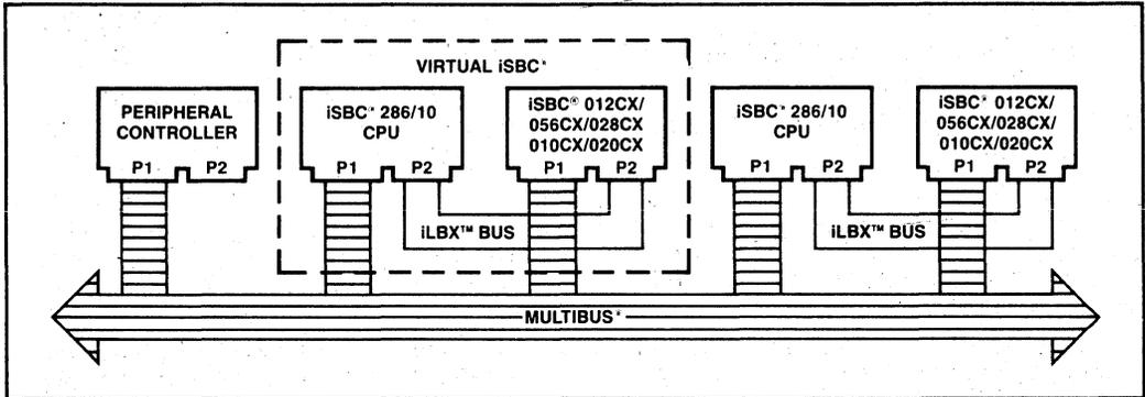
Figure 1. Typical iLBX™ System Configuration
