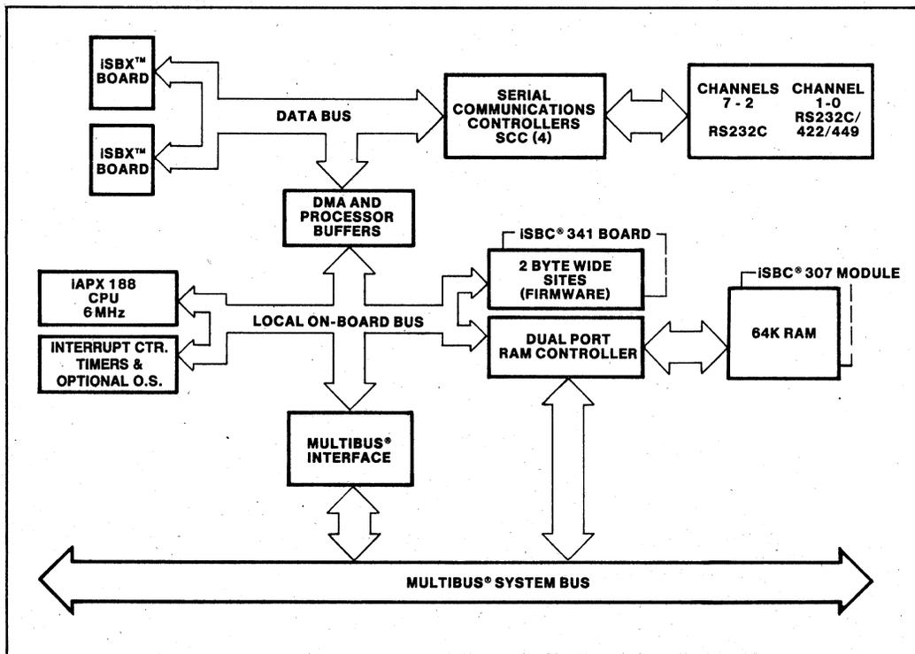
**Figure 4. Block Diagram of iSBC 188/48 Board**
